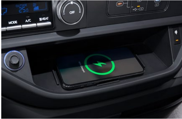
Wireless Charger With 10 W wireless charging, there is no need for charging cables. Safety circuitry automatically shuts off the charging current to prevent your device from overheating.
