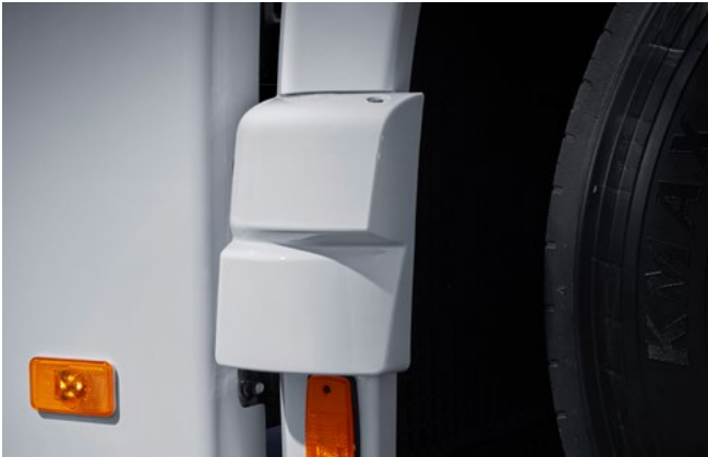
Side-Front Sensor and Side-Rear Sensor Side-front and side-rear sensors enhance safety by detecting blind spots and preventing accidents during reversing and lane changes.
