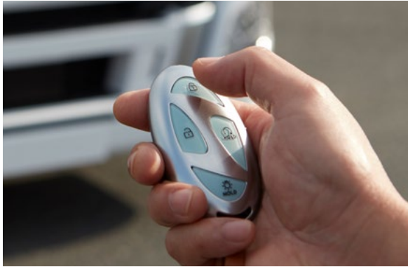
Smart Key The new smart key includes remote start and ECAS operation from outside the vehicle, significantly enhancing operational convenience. *Two keys standard, optional extras available
